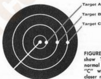
FIGURE 8A: Under abnormal conditions, with cool air overlaid by a warmer air mass, a duct is formed through which the radar pulse travels and reflects Target "C" at a much greater distance.
