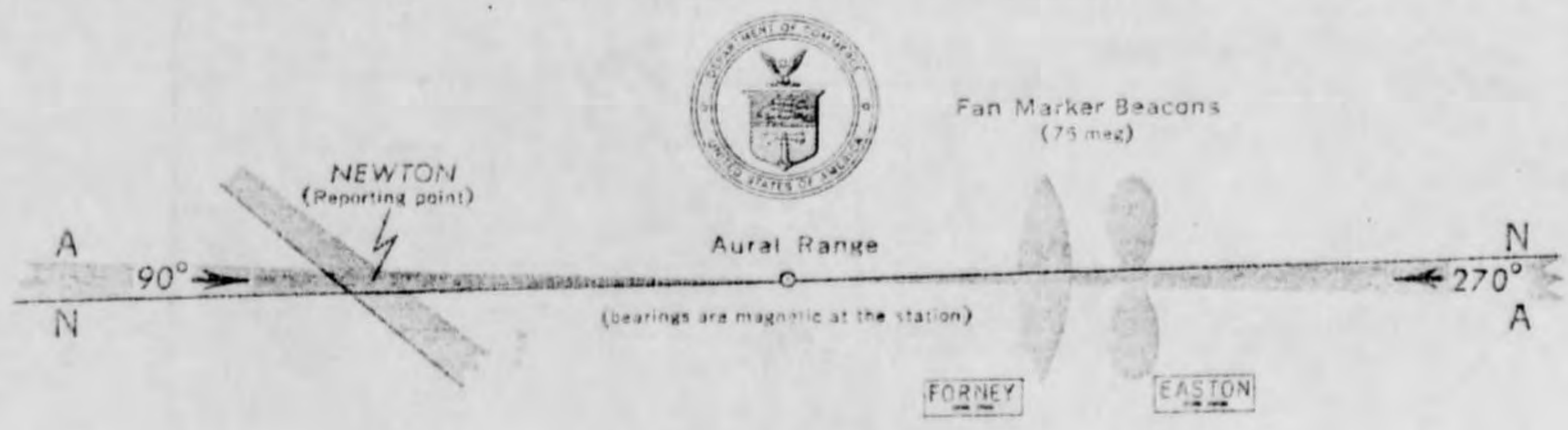
VHF FOUR-COURSE VISUAL-AURAL RADIO RANGE The Blue and Yellow Visual Sectors are indicated by a B and Y; the Aural Sectors by A and N
