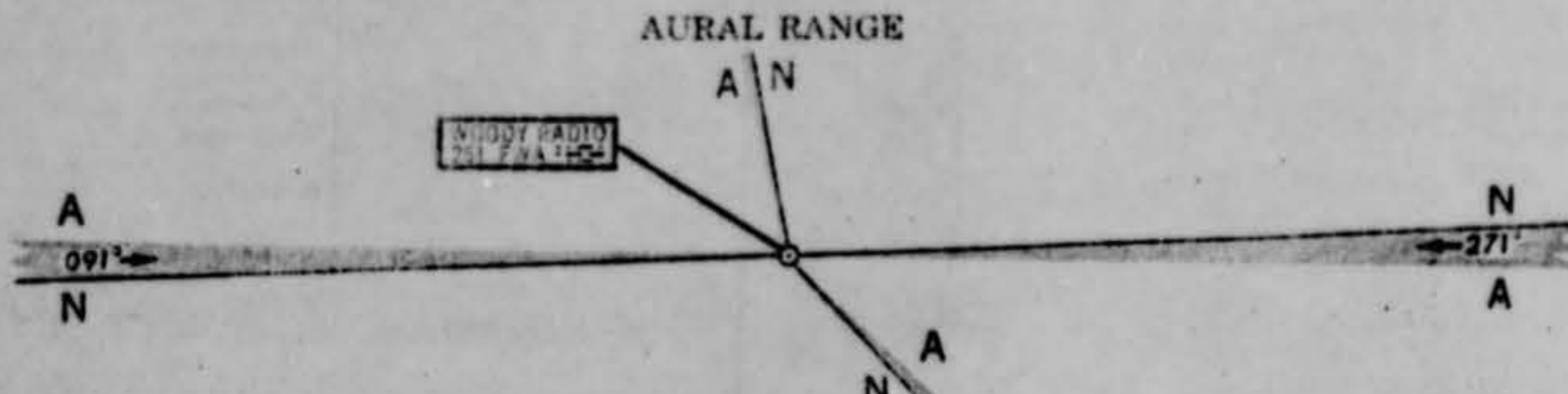
The heavy line indicates the "N" quadrant. The bearings shown are magnetic and the magnetic variation at the position of the ground station is used for computing them.
