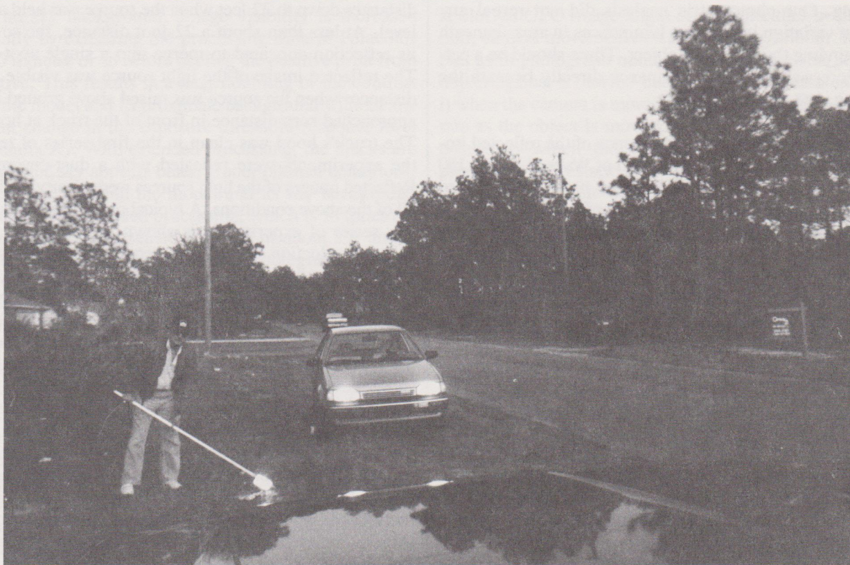
Figure 2: A typical photograph showing reflections in the hood of a Ford 150 XLT truck. The light source at ground-level is 22 feet 4 inches in front of the truck. The automobile headlamps are 29 feet 10 inches away and 25 inches above ground level.
